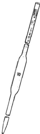
Calibrated to Class A tolerances in accordance with ASTM E-542, and ASTM E-969. Each pipet is individually serialized and supplied with a Certificate of Identification and Capacity, traceable to NIST standards. Sizes 1mL through 25mL are color-coded with colored graduations enameled onto the glass.
