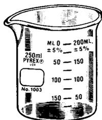
Heavy duty beakers specifically designed to offer the best mechanical strength under harsh conditions, such as mechanized washing operations. For convenience, the 250 through 4000 mL beakers have a double graduated metric scale to indicate their approximate content. All sizes have an extra large marking spot.
