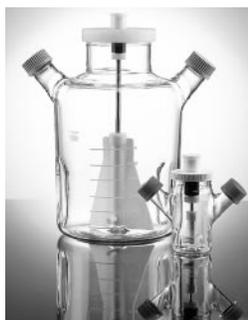
Baffled to enhance agitation of the contents of the flask. Dynamic Vortex impellers ensure high performance stirring. Wide, angled sidearms permit easier entry of 25 mL and 50 mL pipets for feeding and harvesting.
