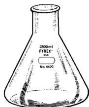
This wide mouth flask is designed for culturing organisms requiring a large surface area to volume ratio. It can also be used in serum production.
