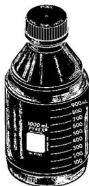
Heavy duty bottle of low actinic glass for use when storing/transporting light sensitive materials. Includes a linerless, one-piece, autoclavable, orange polypropylene, plug-seal cap with drip-free pouring rings. Glass bead indicates full capacity line. Permanent white enamel graduations and marking spots. Thread size: GL45. Neck I.D.: 29 mm I.D.
