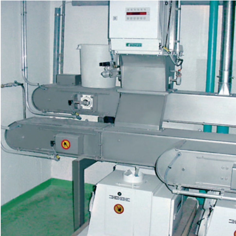
Chain conveyor MNKA. Execution in stainless steel (optional) for top sanitation.
