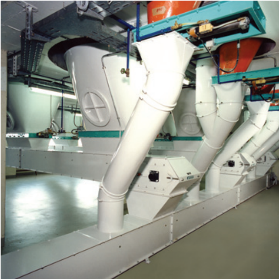
Chain conveyor MNKA. All moving parts completely enclosed for high operational reliability.
